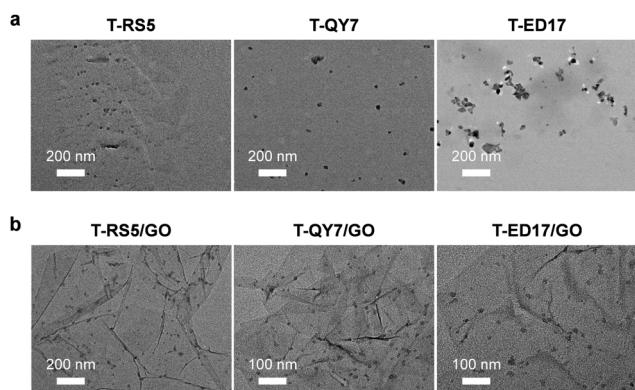
**Fig. 2** Transmission electron microscopic images of (a) **T-RS5**, **T-QY7** and **T-ED17** (10  $\mu$ M), and (b) **T-RS5/GO**, **T-QY7/GO** and **T-ED17/GO** (peptide/GO = 10  $\mu$ M/40  $\mu$ g  $\text{mL}^{-1}$ ).
