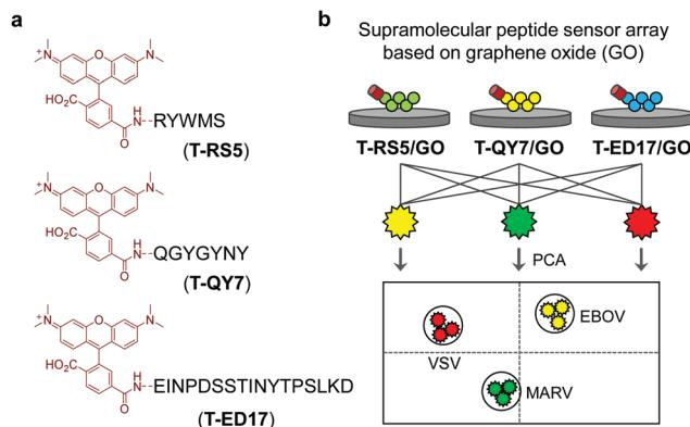
**Fig. 1** (a) Structure of the 5-TAMRA-labeled peptide probes **T-RS5**, **T-QY7** and **T-ED17**. (b) Schematic illustration of the supramolecular fluorogenic peptide sensor array based on graphene oxide (GO) for differential sensing of three viruses including ebola virus (EBOV), marburg virus (MARV) and receptor-extensive vesicular stomatitis virus (VSV) using the principal component analysis (PCA).
