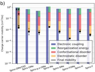
Fig. 5 (a) Simulated and measured hole mobility of spiro-OMeTAD and the spiro-R series, (b) hole mobility of spiro-OMeTAD and the spiro-R and its partitioning in effects of electronic couplings, reorganization energy, conformational disorder and electrostatic disorder.
