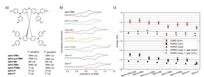
Fig. 4 (a) Definition of the functional groups used for the spiro-R series. (b) Cyclic voltammograms for HTM series recorded in  $0.1 \,\mathrm{M}\,n$ -NBu<sub>4</sub>PF<sub>6</sub> DCM solutions at room temperature. (c) Simulated and experimental HOMO and LUMO energies for the spiro-R series and spiro-OMeTAD as a reference material.
