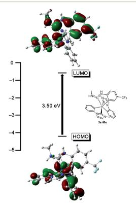
Fig. 7 DFT-computed HOMO and LUMO energy values and plots for the model complex 3a-Me (isovalue = 0.03 a.u.). Calculations were performed in the gas phase at MN15L/6-311G\* for nonmetal atoms, with the SDD basis set used for Ir. The structure of 3a-Me is also shown, in the approximate orientation used for the orbital depictions.
