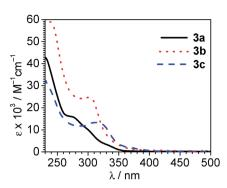
Fig. 4 Overlaid UV-vis absorption spectra of 3a-3c, recorded at room temperature in  $CH_2Cl_2$ .
