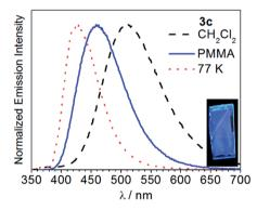
Fig. 5 Photoluminescence spectra of 3a-c recorded in  $CH_2Cl_2$  at room temperature (black trace, dashed line), PMMA film at room temperature (blue trace, solid line), and in 1:3  $CH_2Cl_2$ /toluene glass at 77 K (red trace, dotted line). Samples were excited at  $\lambda=310$  nm. The insets show photographs of the PMMA films under UV illumination.
