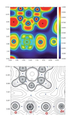
Fig. 9 Electron Localisation Function (ELF) diagram (top) and  $\nabla^2 \rho$  contour line diagram (bottom) of the (py)OUO–Zn fragment in complex 6 (ZnCl) (length unit: Bohr). The value of ELF is given by the colour scale. For the  $\nabla^2 \rho$  diagram, blue points are BCPs, solid lines and dotted lines represent positive and negative values of the Laplacian of the electron density.
