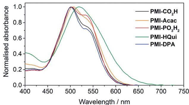
**Fig. 2** UV-Vis spectra of PMI dyes immobilised on a thin TiO<sub>2</sub> film (6  $\mu\text{m}$  thickness) recorded at room temperature.
