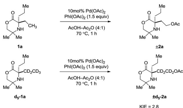
Scheme 3 KIE measured from initial rate comparisons of **1a** and d<sub>5</sub>-**1a**.
