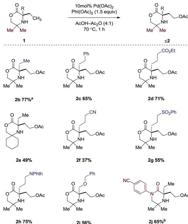
Scheme 5 Scope of acetoxylation of morpholinones. <sup>a</sup> Isolated as a mixture of mono- and diacetoxylation products (1.6 : 1). <sup>b</sup> 15 mol% Pd(OAc)<sub>2</sub> in CH<sub>2</sub>Cl<sub>2</sub>–Ac<sub>2</sub>O (4 : 1).
