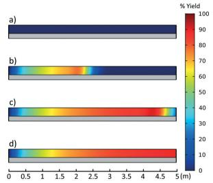
Fig. 4 Percent yield as a function of reactor length at a) 0, b) 0.5, c) 1.0, d) 5.0 times the residence time. Reactor length 5 m, 1 mm ID, 40 °C, 0.1 ml min<sup>-1</sup> flow rate, and 0.95:1 molar ratio. Reactor inlet at left and exiting right. Reactor dimensions not to scale.
