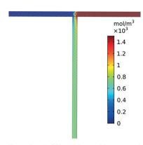
Fig. 3 Three dimensional CFD mixing, without reaction, of 1.5 mol m<sup>-3</sup> of both M4MAA (1) and DMF-DMA (2) entering a tee junction from left and right respectively and exit mixed downward. Pé and Re numbers for this simulation are  $1.51 \times 10^5$  and 5.02 respectively. Red and blue indicate high and low concentrations of DMF-DMA (2) respectively. The dashed line indicates where the reaction was assumed to initiate due to removal of the tee junction.
