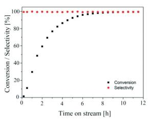
Fig. 11 Catalytic activity and selectivity of semi-continuous dehydrogenation (recycle mode) at a robust set-point, 231.4 °C, 69.3 mL min<sup>-1</sup>  $(464.5 \text{ m}^3 \text{ m}^{-2} \text{ h}^{-1} \text{ at STP}) \text{ nitrogen flow, 0.21 mL min}^{-1} (1.4 \text{ m}^3 \text{ m}^{-2} \text{ h}^{-1})$ at STP) liquid feed flow and 9.28 wt% substrate concentration as a function of stream time (h).
