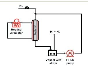
**Fig. 10** The simplified scheme of semi-continuous dehydrogenation (recycle mode) of 1,4-cyclohexanedione.
