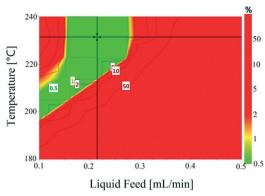
**Fig. 9** Design space for the conversion of 1,4-cyclohexanedione in single-pass mode as a function of temperature (180–240 °C) and liquid feed flow (0.1–0.5 mL min<sup>-1</sup>, 0.7–3.3 m<sup>3</sup> m<sup>-2</sup> h<sup>-1</sup> at STP). The green area is the operating window to meet the desired specification, with the red area indicating risk of failure.
