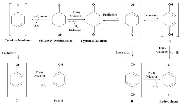
Scheme 1 Reaction schematic for dehydrogenation of 1,4-cyclohexanedione and formation of 4-hydroxycyclohexanene and phenol by-products.
