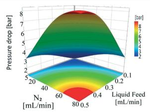
Fig. 5 Influence of nitrogen flow (5–80 mL  $min^{-1}$ , 33.3–566.7  $m^3$   $m^{-2}$  $h^{-1}$  at STP) and liquid feed flow (0.1–0.5 mL min<sup>-1</sup>, 0.7–3.3 m<sup>3</sup> m<sup>-2</sup>  $h^{-1}$ at STP) on the pressure drop for a substrate concentration of 1 wt% at 220 °C, in single-pass mode.
