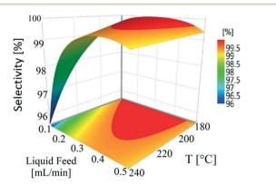
Fig. 4 Influence of temperature (180-240 °C) and liquid feed flow  $(0.1-0.5 \text{ mL min}^{-1}, 0.7-3.3 \text{ m}^3 \text{ m}^{-2} \text{ h}^{-1} \text{ at STP})$  on the conversion and selectivity of 1,4-cyclohexanedione for a fixed nitrogen flow (40 mL min<sup>-1</sup>, 266.4 m<sup>3</sup> m<sup>-2</sup> h<sup>-1</sup> at STP) and substrate concentration (10 wt%) in single-pass mode.
