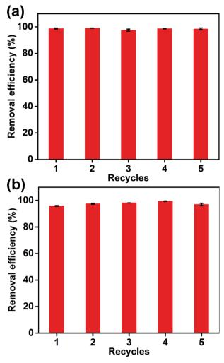
Fig. 11 Removal efficiencies for (a) MB and (b) CV were >95% after five Dex-MA/PAA hydrogel adsorption/desorption cycles. Dex-MA/PAA hydrogel dose:  $1 \text{ q L}^{-1}$ , dye concentration:  $50 \text{ mg L}^{-1}$ ,  $pH_{\text{initial}}$  8.0.
