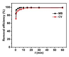
Fig. 8 Effect of contact time, t, on the dye removal efficiency. Hydrogel adsorbent dose: 1 g L<sup>-1</sup>, dye concentration: 50 mg L<sup>-1</sup>, pH<sub>initial</sub> 8.0.
