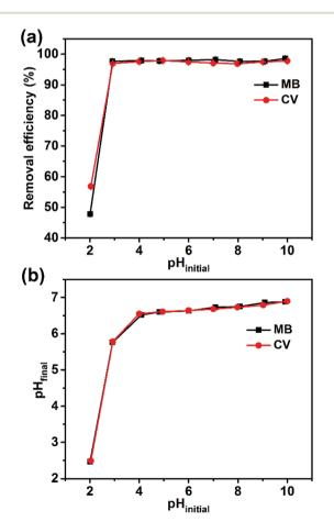
Fig. 5 (a) Effect of initial solution pH on the removal efficiency by the Dex-MA/PAA hydrogel and (b) finial pH changes after adding the Dex-MA/PAA hydrogel. Dex-MA/PAA hydrogel dose:  $1~{\rm g~L}^{-1}$ , dye concentration:  $50~{\rm mg~L}^{-1}$ , contact time:  $3~{\rm h.}$
