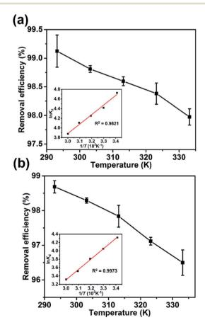
Fig. 7 The effect of temperature on the removal efficiency: (a) MB and (b) CV (inset: Van't Hoff plots for the adsorption of MB and CV on Dex-MA/PAA).
