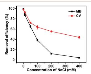
Fig. 6 Effect of NaCl concentration on removal efficiency of Dex-MA/PAA hydrogel (Dex-MA/PAA hydrogel dose:  $1 \text{ g L}^{-1}$ , dye concentration: 50 mg L<sup>-1</sup>, contact time: 3 h, initial pH 8.0).
