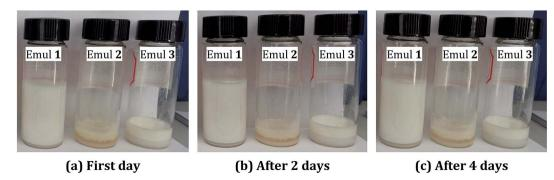
Fig. 2 The optical images of emulsions at different storage times. (a) On first day. (b) After 2 days. (c) After 4 days.
