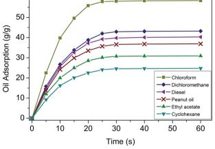
Fig. 6 (a) Oil adsorption of foams with different amounts of water; (b) adsorption kinetics of foams.
