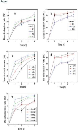
Fig. 2 Decolorization rate of simulated wastewater under different conditions. (a) Inoculation ratio of XJ-2 and XJK; (b) inoculation time of XJ-2; (c) pH; (d) temperature; (e) rotation speed of shaker.
