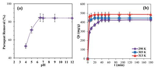
Fig. 4 (a) Effect of initial solution pH (T = 298 K;  $C_i = 100 \text{ mg L}^{-1}$ ; m = 20 mg). (b) Effect of contact time (temperature: 298, 303, and 313 K;  $C_i = 100 \text{ mg}$ ). 100 mg L<sup>-1</sup>; m = 20 mg; pH = 6.5).
