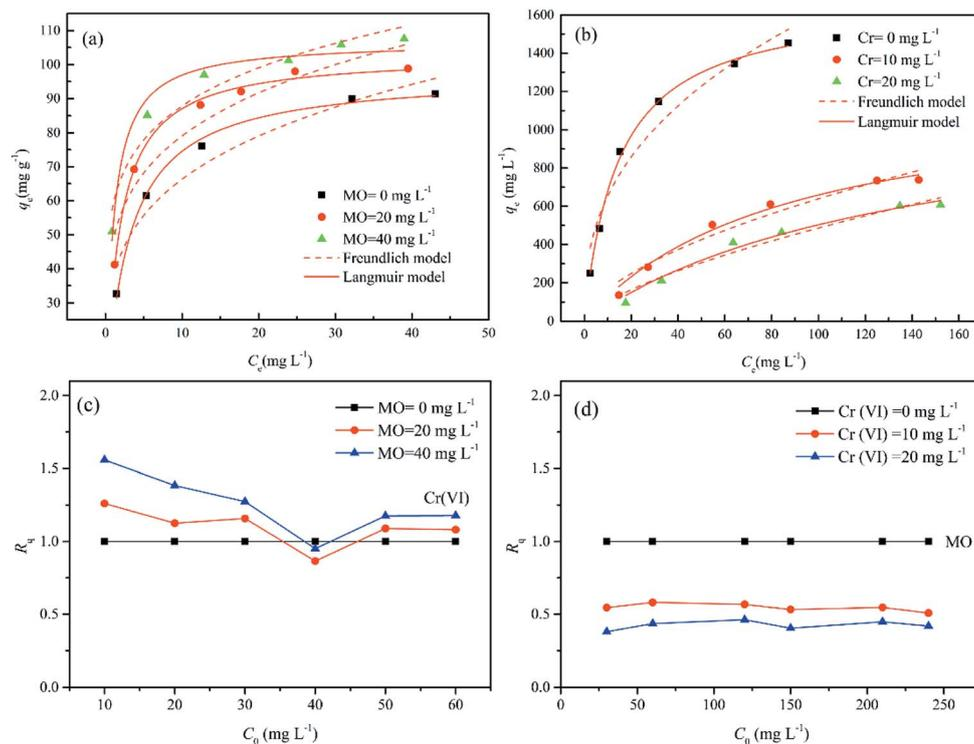
Fig. 6 Adsorption isotherms of Cr(vi) (a) and MO (b) by MWCNTs@Fe<sub>3</sub>O<sub>4</sub>/PEI in MO-Cr(vi) binary system. (Conditions: initial dye concentration, 30–240 mg L<sup>-1</sup> for MO, 10–60 mg L<sup>-1</sup> for Cr(vi); adsorbent dosage, 3 mg for MO, 10 mg for Cr(vi); solution pH, 3; contact time, 6 h for MO, 4 h for Cr(vi); temperature, 25–55 °C; and agitation speed, 150 rpm.)
