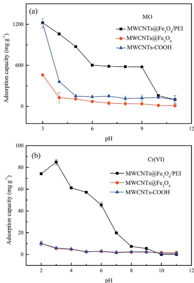
Fig. 3 Effect of solution pH on uptake of MO (a) and Cr(vi) (b) by different adsorbents (conditions: initial dye concentration, 200 mg L<sup>-1</sup> for MO, 50 mg L<sup>-1</sup> for Cr(vi); adsorbent dosage, 3 mg for MO, 10 mg for Cr(vi); solution pH, 3–11; contact time, 6 h; temperature, 25 °C; and agitation speed, 150 rpm).
