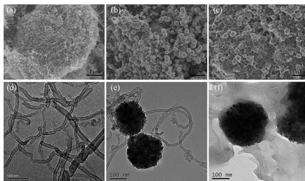
Fig. 1 SEM images of MWCNTs (a), MWCNTs@Fe<sub>3</sub>O<sub>4</sub> (b), MWCNTs@Fe<sub>3</sub>O<sub>4</sub>/PEI (c), and TEM images of MWCNTs (d), MWCNTs@Fe<sub>3</sub>O<sub>4</sub> (e), MWCNTs@Fe<sub>3</sub>O<sub>4</sub>/PEI (f).
