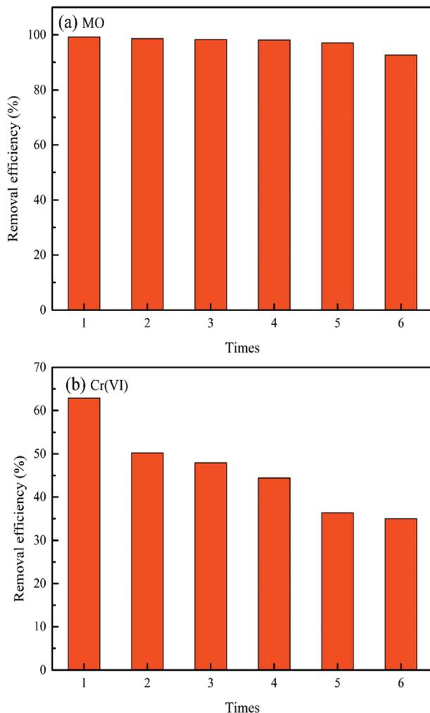
Fig. 5 Regeneration and stability studies of MO and Cr(vi) on MWCNTs@Fe<sub>3</sub>O<sub>4</sub>/PEI with six cycles (conditions: initial dye concentration, 200 mg L<sup>-1</sup> for MO, 50 mg L<sup>-1</sup> for Cr(vi); adsorbent dosage, 15 mg; solution pH, 3; contact time, 6 h for MO, 4 h for Cr(vi); temperature, 25 °C; and agitation speed, 150 rpm).
