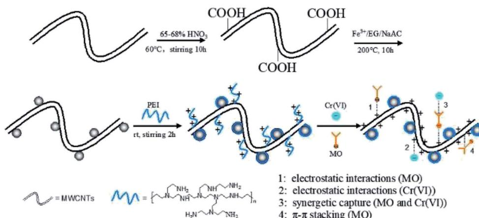
Scheme 1 Synthesis of MWCNTs@Fe<sub>3</sub>O<sub>4</sub>/PEI composite and the proposed adsorption mechanisms.
