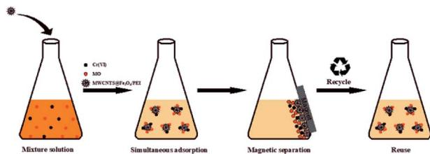
Scheme 2 Schematic diagram for simultaneous capture of MO and Cr(vi) in MO-Cr(vi) binary system.
