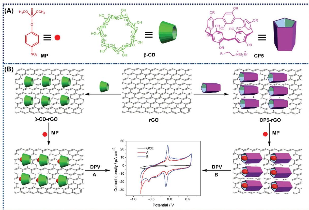
Fig. 1 The corresponding cartoon representations of MP, CP5 and  $\beta$ -CD and the illustration of CP5-rGO (A) and  $\beta$ -CD-rGO (B) nanohybrids-based electrochemical sensing method towards methyl parathion.
