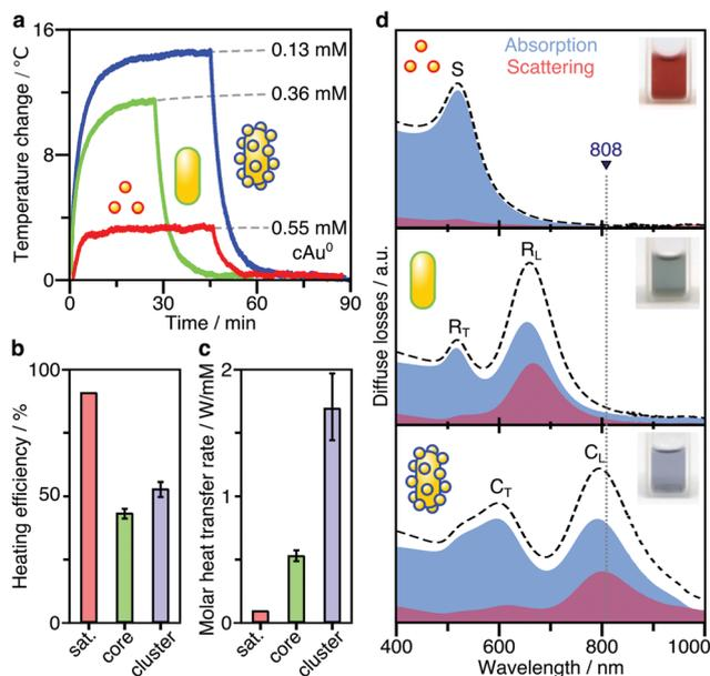
**Fig. 5** Plasmonic heating efficiency: (a) Exemplary heating/cooling cycles of assemblies (blue) and building blocks (green: rods; red: spheres). Heating efficiency (b) and molar rate of heat transfer (c) for excitation at 808 nm. (d) Spectral losses measured by diffuse reflectance spectroscopy of the spherical satellites (top), the rod-shaped cores (middle), and the assemblies (bottom) showing non-radiative (blue) and radiative contributions (red) to the total extinction (black, dashed).
