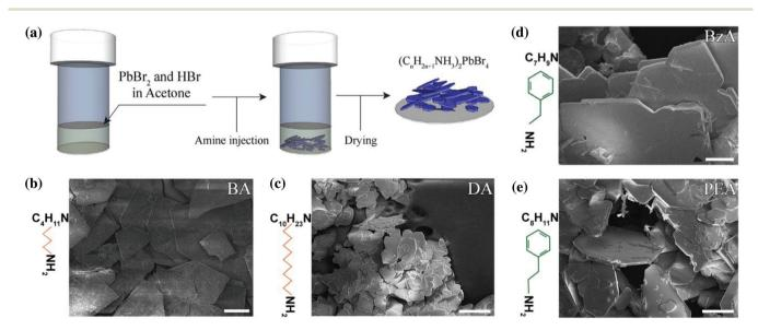
Fig. 1 (a) Schematic diagram of the facile fabrication process of the layered perovskite by injecting a primary amine to a mixture of PbBr2 in HBr and acetone. (b-e) SEM images of the produced platelets when using short and long aliphatic molecules, such as butylammonium (BA) (b) and decylammonium (DA) (c), and aromatic ones as benzylammonium (BzA) (d) and phenethylammonium (PEA) (e). Scale bars: 100 µm.
