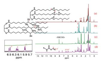
Fig. 3 <sup>1</sup>H NMR spectra of (a) pure soybean oil (ESO), (b) methoxylated soybean oil-based polyol (MESO), (c) MNCO (MESO reacted with isophorone diisocyanate), and (d) RWPU.
