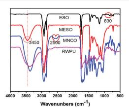
Fig. 2 FTIR spectra of pure soybean oil (ESO), methoxylated soybean oil-based polyol (MESO), MNCO (MESO reacted with isophorone diisocyanate), and RWPU.
