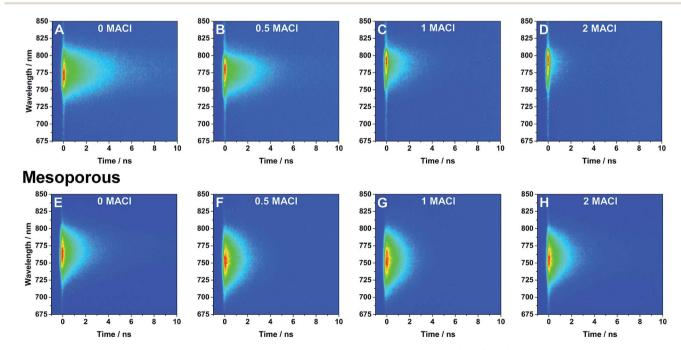
Fig. 3 TRPL spectra of perovskite films with various ratios of MACl precursor (noted in figure) on (A-D) planar and (E-H) mesoporous  $TiO_2$  excited using 480 nm light.
