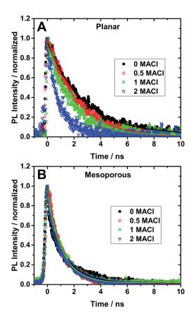
Fig. 4 TRPL decay dynamics (symbols) and their fits (lines) of perovskite films on (A) planar  ${\rm TiO_2}$  and (B) mesoporous  ${\rm TiO_2}$  coated FTO substrates excited using 480 nm light. The lifetimes obtained from the single exponential fits are reported in Table 1.
