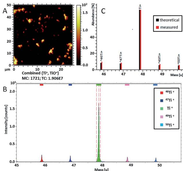
Fig. 4 Results of ToF-SIMS analysis of  $\text{TiO}_2$  NPs in delayed extraction mode. (A) Lateral yield distribution overlay of representative Ti-containing secondary ion species. (B) Measured isotopic distribution of  $\text{Ti}^+$ , all isotopes of titanium are clearly visible in the spectra and are in agreement with the natural abundance pattern as shown in (C).
