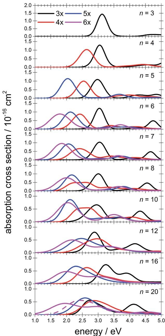
Fig. 2 Calculated spectra of selected  $[\text{Mg}(\text{H}_2\text{O})_n]^+$  ions with different Mg coordination numbers ( $3x-6x$ ). Calculated at the CAM-B3LYP/aug-cc-pVDZ// $\omega$ B97XD/def2TZVP level of theory using the linearized reflection principle to calculate the peak width. Surface and inner isomers for  $n = 20$  are shown with full and dashed lines, respectively. Benchmarking with respect to the ADC(2) method can be found in Fig. S4.†
