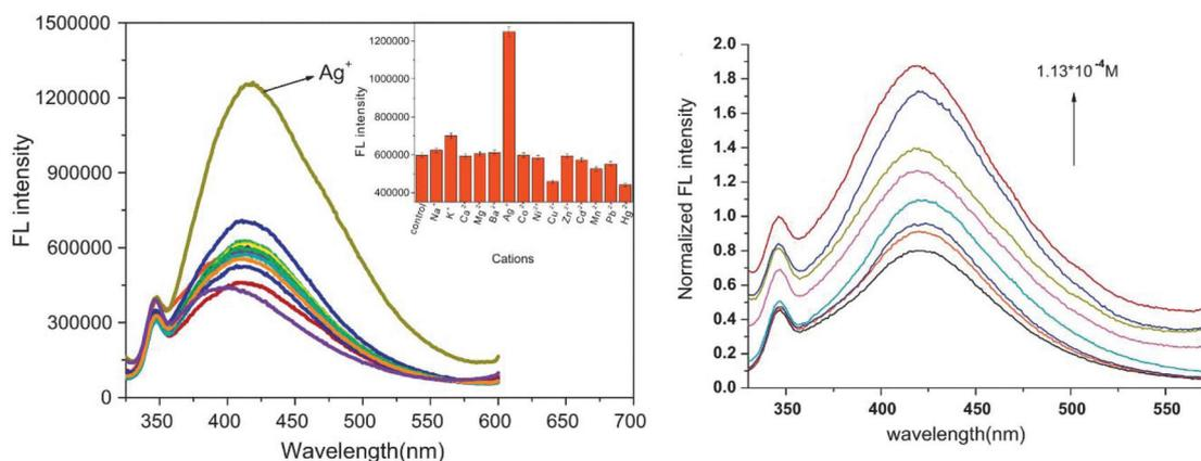
Fig. 2 Fluorescence emission spectra of FONs ( $7.5 \times 10^{-6}$  M) with or without various cations and plot of the fluorescent intensity as a function of  $\text{Ag}^+$  concentration. Adapted with permission from ref. 46. Copyright 2011 Elsevier Ltd.
