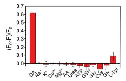
Fig. 4 Relative fluorescence decrement  $((F_0 - F)/F_0)$  of the bioprobe (15  $\mu$ g mL<sup>-1</sup>) in the presence of different interfering substances.  $F_0$ : Fluorescence intensity of the blank, F: fluorescence intensity of the bioprobe upon the addition of the inspected species. Dopamine: 10 µM,  $Na^+/K^+$ : 1 mM, L-Tyr: 10  $\mu$ M, other substances: 100  $\mu$ M.
