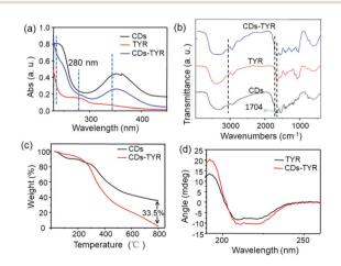
**Fig. 2** (a) UV-Vis spectra of CDs, TYR and CDs-TYR, respectively; (b) FT-IR spectra of CDs, TYR and CDs-TYR; (c) TGA curves of CDs and CDs-TYR; (d) CD spectra of TYR before (black line) and after (red line) the conjugation with CDs.
