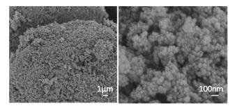
Fig. 3 SEM images of the un-doped VO<sub>2</sub>(M) powder.
