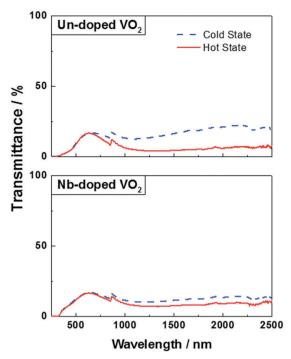
Fig. 9 UV-Vis spectra of un-doped VO<sub>2</sub> (top) and Nb-doped VO<sub>2</sub> (bottom) at 20 °C (blue dashed line) and 90 °C (continuous red line).
