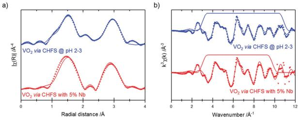
Fig. 7 VK-edge Fourier transforms (a) and EXAFS (b) of the CHFS VO<sub>2</sub> samples. Data are plotted as symbols, and fits as solid lines. The trapezoid lines in (b) indicate the Fourier transform window used.
