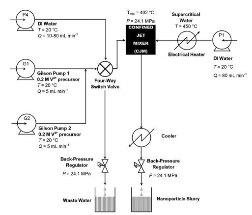
Fig. 1 Schematic diagram of the continuous hydrothermal flow synthesis (CHFS) process used in the direct synthesis of VO<sub>2</sub>(M) nanoparticles.
