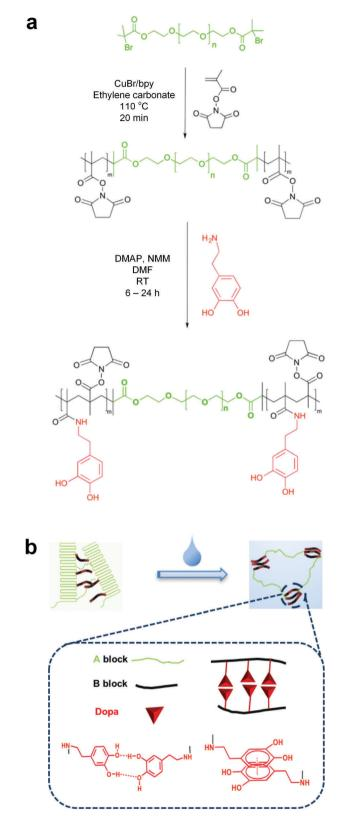
Fig. 1 Design and processing of precursor. (a) Schematic showing the synthesis of poly(NHSMA)-b-PEG-b-poly(NHSMA) (ABA-Dopa(-)) and poly(NHSMA)-b-PEG-b-poly(NHSMA)-Dopa (ABA-Dopa(+)) triblock copolymers. (b) Schematic illustration of polymer processing to create the hydrated ABA-Dopa(+) network.
