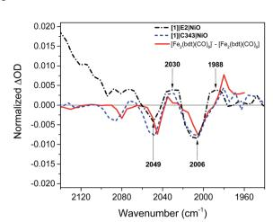
Fig. 5 Comparison of the IR transient absorption spectrum of the [1]| E2|NiO film 1 ps after excitation at 532 nm (black), the [1]|C343|NiO film 1 ps after excitation at 440 nm (blue), and the IR transient absorption spectrum of [Fe<sub>2</sub>(bdt)(CO)<sub>6</sub>] $^-$ -[Fe<sub>2</sub>(bdt)(CO)<sub>6</sub>] obtained by reduction of [Fe<sub>2</sub>(bdt)(CO)<sub>6</sub>] with flash-quench generated [Ru(dmb)<sub>3</sub>] $^+$  (ref. 18) (red).
