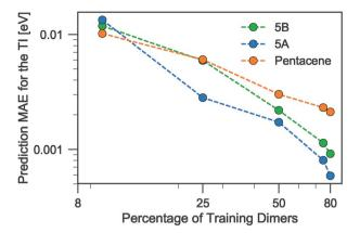
Fig. 7 Learning curves for the MAE in predicting TI when using FPS selection of the training set. The three systems are compared as a function of the fraction of the total symmetry-independent dimer configurations.
