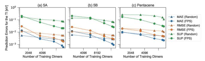
Fig. 6 Learning curves for the errors in predicting TI when selecting training dimers using a random or FPS strategy. MAE, RMSE and SUP errors are defined in the text.
