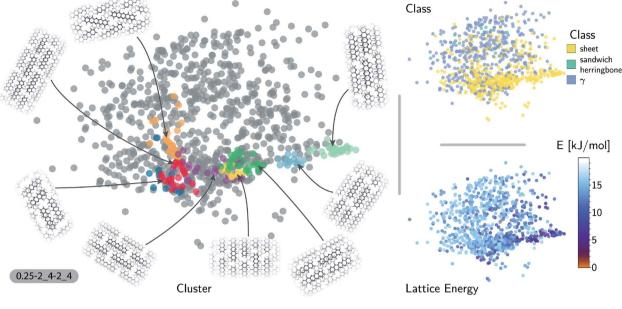
Fig. 5 Representation of the similarity matrix for 5B. The atomic configurations, *i.e.* disks, on the three sketch-maps are color-coded according to their lattice energy (bottom right), class following the heuristic classification (top right) and cluster index (gray structure do not belong to a cluster) found using HDBSCAN\* on the similarity matrix (left). The structural pattern of each cluster is illustrated with a top view of the 5B polymorphs.
