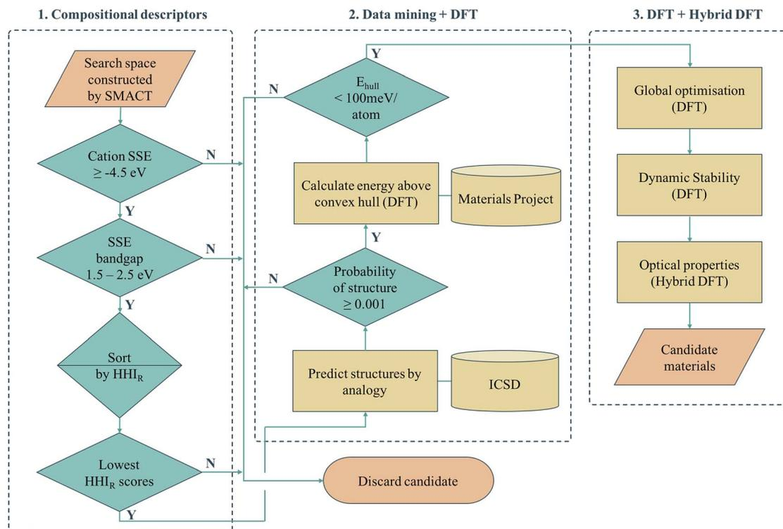
Fig. 1 Computer-aided-design workflow used for exploring novel photoactive semiconductors. *SMACT* refers to our screening package, SSE refers to the solid-state energy scale,  $HHI_R$  refers to the Herfindahl–Hirschman Index for sustainability, while DFT refers to density functional theory.
