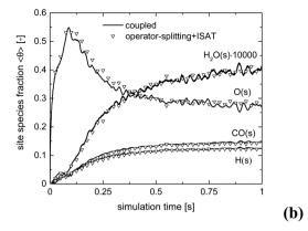
Fig. 10 Comparison of the average compositions for the isothermal CPO process, derived with the coupled approach and operator-splitting + ISAT: species mass fraction (a) and relevant species site fractions (b).
