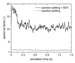
Fig. 8 Chemical speed-up factors obtained with the operator-splitting and the operator-splitting + ISAT techniques as a function of time for the isothermal methane steam reforming process.
