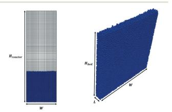
Fig. 2 Computational grid (on the left) and initial packed bed geometry (on the right) of the test cases.  $H_{reactor}$ , W and L are the reactor height, width and depth, respectively, whereas  $H_{\text{bed}}$  is the height of the initial packed bed configuration.
