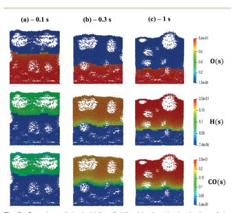
Snapshot of the bubbling fluidized bed at the beginning of the simulation at t = 0.1 s (a), during the syngas production at t = 0.3 s (b) and the pseudo-steady state at t = 1 s (c), simulated with the operating conditions listed in Table 1 for the methane CPO. The catalytic bed is represented reporting each catalytic particle as a sphere. The catalytic pellets are mapped as a function of their O, H and CO site fraction. Particle-free regions represent the bubbles of gas.
