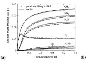
Fig. 5 Comparison of the average mass fraction composition for the isothermal CPO process, derived with: coupled approach and operator-splitting (a) and coupled approach and operator-splitting + ISAT (b).
