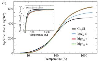
Fig. 4 (a) Phonon partial density of states and derivative of the phonon occupation functions of the  $\text{Cu}_2\text{Si}$  monolayer and its hydrogenated derivatives at various temperatures. Red, light and dark blue lines represent the functions calculated at 1000, 300, and 20 K. (b) For the  $\text{Cu}_2\text{Si}$  monolayer and its hydrogenated derivatives, constant volume specific heat per mass is demonstrated as a function of temperature in logarithmic scale.
