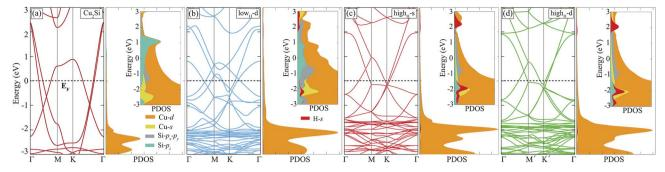
Fig. 5 Electronic band structure and PDOS are demonstrated for monolayers of (a)  $Cu_2Si$ , (b)  $low_H-d$ , (c)  $high_H-s$ , and (d)  $high_H-d$ . Fermi level,  $E_F$ , is set to zero. Inset figures of PDOS are rescaled with respect to the number of atoms per unit cell.
