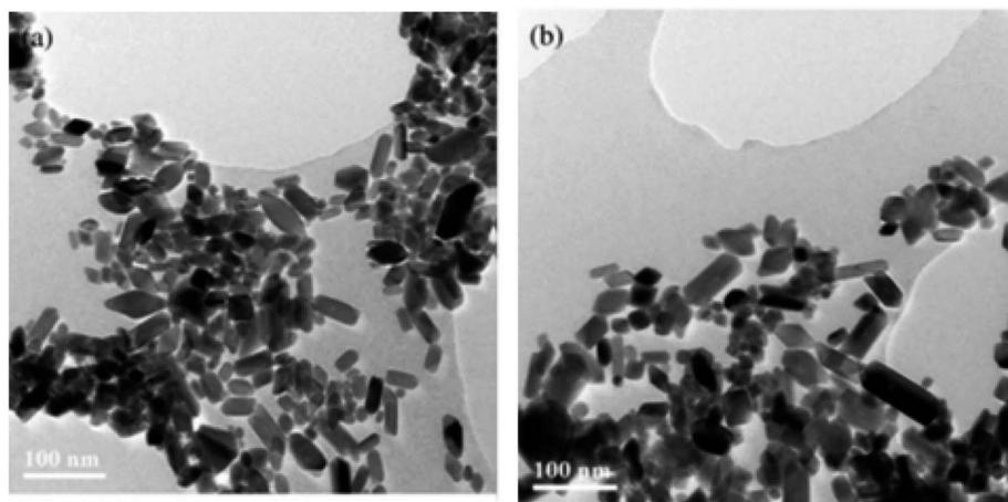
Fig. 7 TEM images of TiO<sub>2</sub> nanoparticles after hydrothermal treatment of TBA peptized gel at (a) 210 °C and (b) 270 °C.<sup>133</sup>
