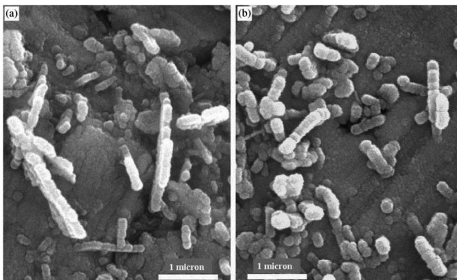
Fig. 14 SEM micrograph of  $\text{TiO}_2$  nanowires deposited without  $\text{NH}_3$  at  $500^\circ\text{C}$ ; (a) with 800 sccm argon flow, and (b) with 500 sccm argon flow.<sup>163</sup>
