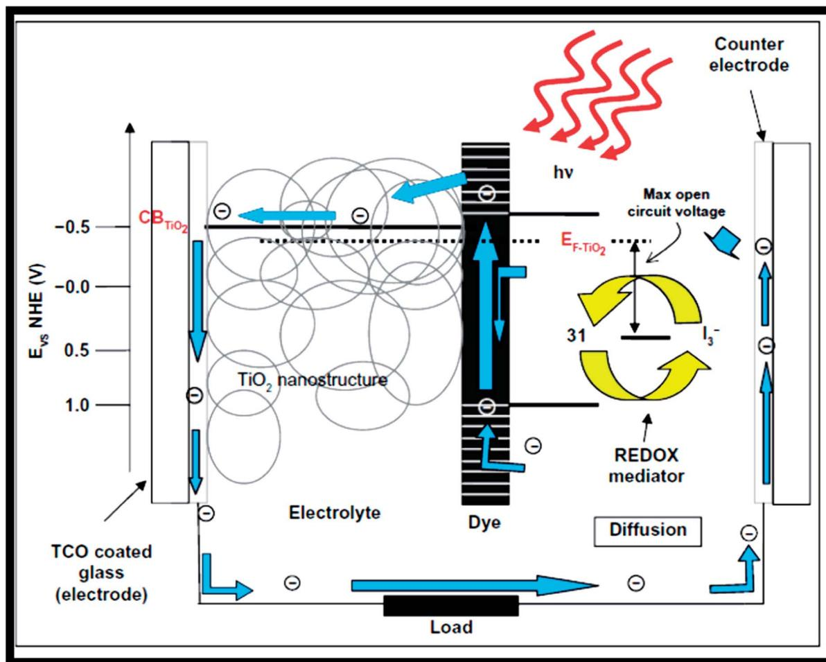
Fig. 16 Operation principles and energy levels of nanocrystalline dye-sensitized solar cell.<sup>41</sup>
