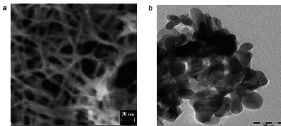
Fig. 9 Electron microscopy images of (a) titania powders and (b) titania nanotubes.<sup>312</sup>
