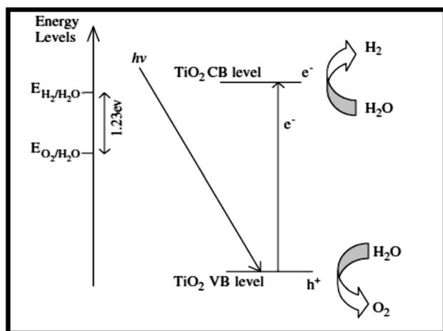
Fig. 17 Mechanism of  $\text{TiO}_2$  photocatalytic water-splitting for hydrogen production.<sup>230</sup>
