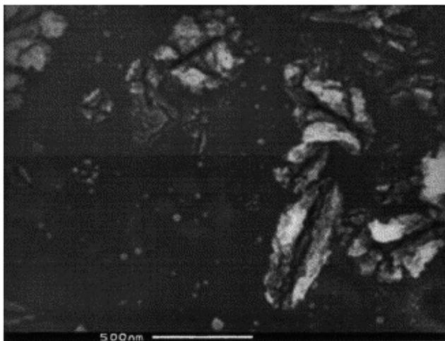
Fig. 12 Scanning electron micrograph of TA6V anodised in CA electrolyte.<sup>144</sup>
