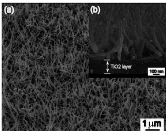
Fig. 15 SEM images of the  $\text{TiO}_2$  nanowire arrays prepared by the PVD method.<sup>176</sup>
