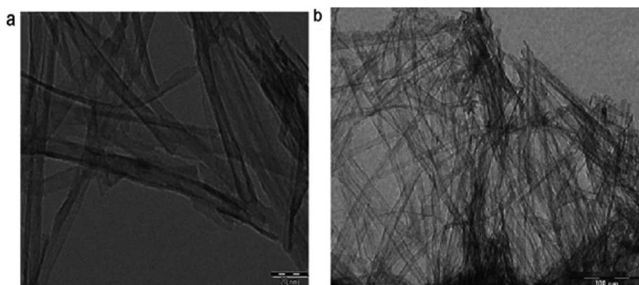
Fig. 10 TEM images of titania nanotubes at (a) low magnification and (b) high magnification.<sup>338</sup>
