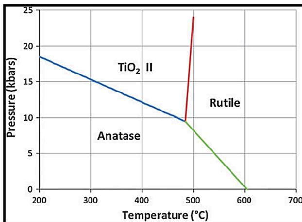
Fig. 3 Reaction boundaries of phase transitions in  $\text{TiO}_2$ .<sup>74</sup>
