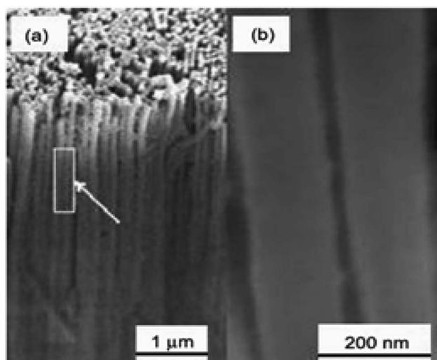
Fig. 6 SEM of TiO<sub>2</sub> nanorods growth in AAM template, (a) low magnification image, (b) high magnification image.<sup>123</sup>
