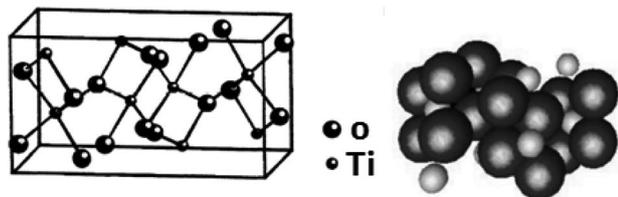
Fig. 2 Lattice structure of brookite  $\text{TiO}_2$ .
