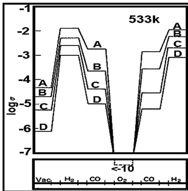
Fig. 4 Influence of gas cycle of sequence on electrical conductivity of 0.5% Pt/ $\text{TiO}_2$  doped with (A)  $\text{W}^{6+}$  (B)  $\text{Ta}^{5+}$  (C) undoped and (D)  $\text{Mg}^{2+}$ .<sup>85</sup>
