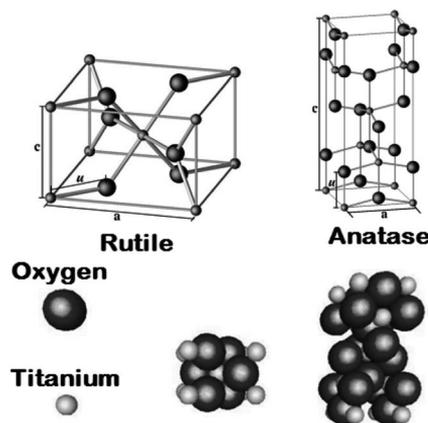
Fig. 1 Crystal structures of the rutile and anatase phases of TiO<sub>2</sub>. Small spheres represent Ti atoms, large spheres represent oxygen atoms.
