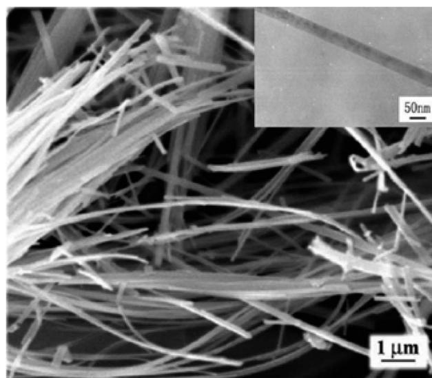
Fig. 8 SEM images of TiO<sub>2</sub> nanowires and a TEM image of a single nanowire prepared by Zhang and colleagues.<sup>135</sup>
