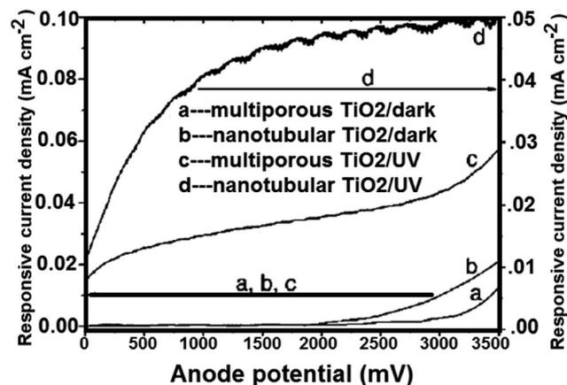
Fig. 18 Measured current of crystallized porous and nanotubular  $\text{TiO}_2/\text{Ti}$  electrodes under linearly swept potential from 0 to 3500 mV vs. SEC.<sup>217</sup>
