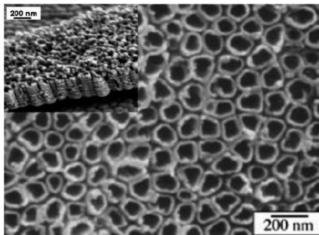
Fig. 13 SEM images of  $\text{TiO}_2$  nanotubes prepared with anodic oxidation.<sup>159</sup>
