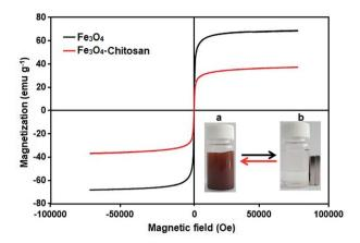
Fig. 11 VSM measurements of the obtained  $Fe_3O_4$  and  $Fe_3O_4$ -chitosan particles. The photographic image of  $Fe_3O_4$ -chitosan particles (a) without magnet and (b) with magnet.
