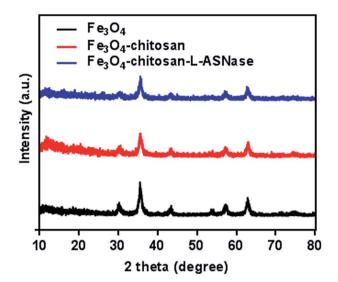
Fig. 7 XRD patterns of the  $Fe_3O_4$ ,  $Fe_3O_4$ -chitosan particles, and  $Fe_3O_4$ -chitosan-L-ASNase.
