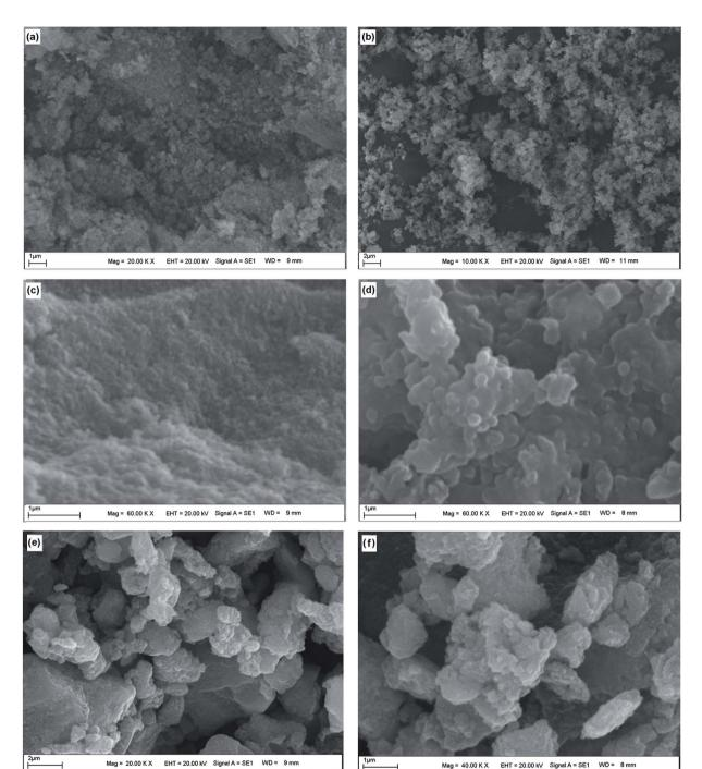
Fig. 9 SEM analysis of magnetic (a and c)  $Fe_3O_4$ , (b and d)  $Fe_3O_4$ -chitosan particles and (e and f)  $Fe_3O_4$ -chitosan-L-ASNase at different magnifications.
