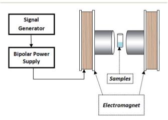
Fig. 2 Schematic of magnetic field experiments(VSM).
