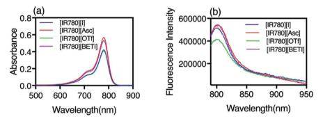
(a) Absorbance spectra and (b) fluorescence emission spectra of IR780 and IR780-based GUMBOS in acetonitrile
