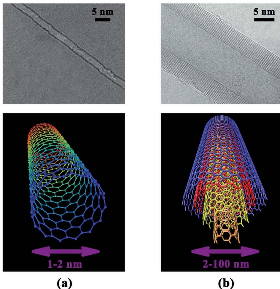
**Fig. 1** Transmission electron microscopy images and schematic diagrams of carbon nanotubes, showing typical diameters of (a) a single-walled carbon nanotube and (b) a multi-walled carbon nanotube. The microscopy image of the single-walled carbon nanotube is adapted with permission from ref. 5. Copyright 2012, Springer Nature Limited. The microscopy image of the multi-walled carbon nanotube is adapted from the "Endo Laboratory" website.<sup>6</sup>
