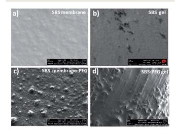
Fig. 5 SEM images of (a) SBS membrane (scale bar 1  $\mu$ m) (b) SBS gel (scale bar 1  $\mu$ m) (c) SBS membrane-PEG (scale bar 2  $\mu$ m) and (d) SBS-PEG gel (scale bar 2  $\mu$ m). SBS membrane-PEG gels were prepared by casting SBS solution after incorporation of PEG particles. SBS gel and SBS-PEG gel were prepared by crosslinking of SBS solution after incorporation of PEG particles. Hybrid gels were dried in vacuum oven overnight before analysis with SEM.
