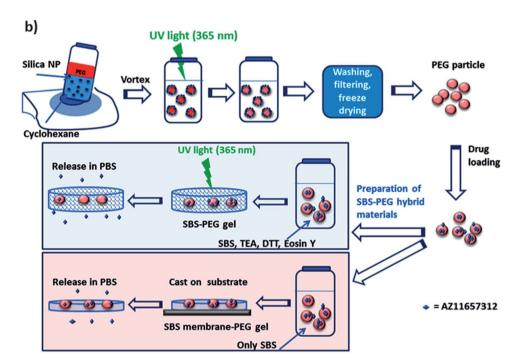
Scheme 1 (a) Components of amphiphilic and crosslinked SBS-PEG gel network, (b) summary of preparation steps for the synthesis of SBS-PEG and SBS membrane-PEG
