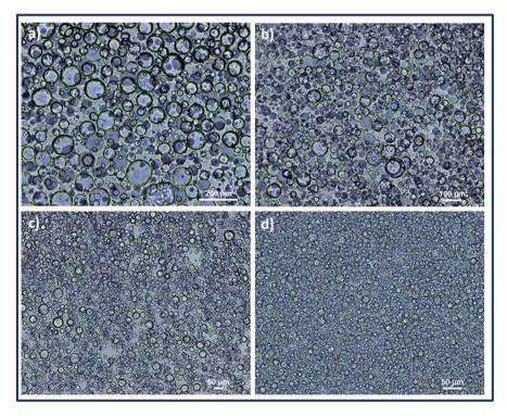
Fig. 2 Light microscope images of PEG-cyclohexanone ( $\varphi = 0.25$ ) water in oil silica nanoparticle (1.5%) stabilized Pickering emulsions prepared by vortex times of (a) 30 s, (b) 60 s, (c) 2 min, (d) 8 min.
