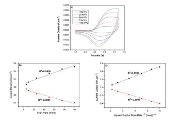
Fig. 3 (a) Cyclic voltammogram of PEDOT nanofibers in 0.1 M NBu<sub>4</sub>PF<sub>6</sub>/ACN at various scan rates, and plots of the anodic and cathodic peak current densities vs. (b) the scan rate, (c) the square root of the scan rate
