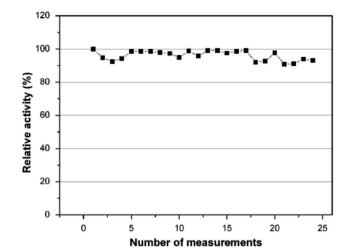
Fig. 8 Operational stability of the PEDOT-NFs/GOx-3 biosensor.
