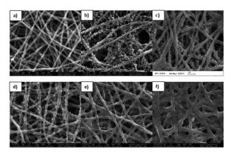
Fig. 4 SEM images of (a) PEDOT nanofibers in phosphate buffer, (b) a PEDOT-NFs/GOx-1 nanofiber mat, (c) a PEDOT-NFs/GOx-2 nanofiber mat, (d) a PEDOT-NFs/GOx-3 nanofiber mat, (e) a PEDOT-NFs/GOx-4 nanofiber mat and (f) a PEDOT-NFs/GOx-5 nanofiber mat. (The magnification is  $15\,000\times$ ).
