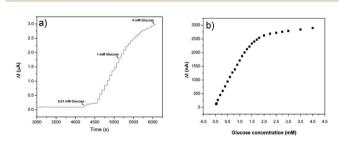
Fig. 6 (a) Amperometric response of the PEDOT-NFs/GOx-3 biosensor to the addition of glucose and (b) the calibration curve of the PEDOT-NFs/GOx-3 biosensor at 0.6 V, pH: 6.5.
