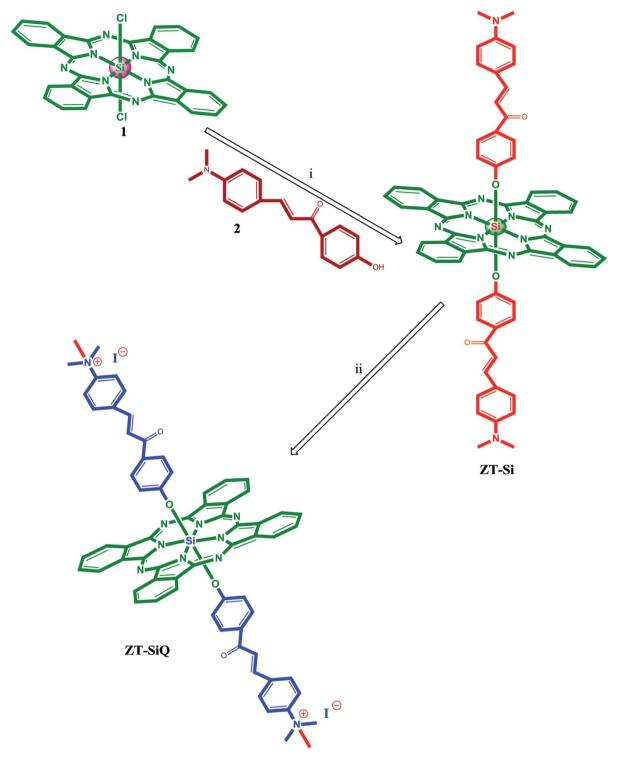
Fig. 2 The synthesis of the silicon(v) phthalocyanine ZT-Si and its quaternized derivative ZT-SiQ. (i) Toluene, NaH, reflux. (ii) CHCl<sub>3</sub>, CH<sub>3</sub>-I, room temperature.
