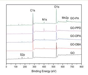
Fig. 8 XPS survey spectra of GO and GO-amine samples.
