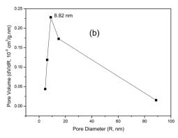
Fig. 3  $N_2$  adsorption-desorption isotherm for GO: (a) BET surface area measurement and (b) BJH pore size distribution.
