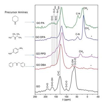
Fig. 7 <sup>13</sup>C NMR spectra of GO and GO-amines. The asterisks indicate spinning sidebands.
