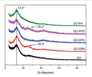
Fig. 1 XRD patterns of GO, GO-DBA, GO-DPA, GO-PPD and GO-PA.
