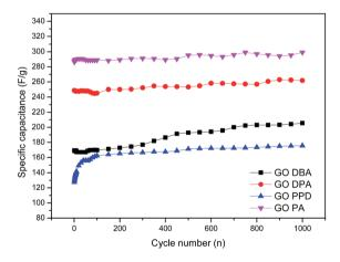
Fig. 13 Cyclic stability tests for the amine-functionalized electrodes at 1 mA  $\rm cm^{-2}$  discharge current density in aqueous 1.0 M  $\rm H_2SO_4$  electrolyte solution.
