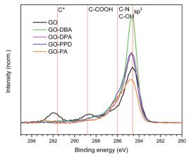
Fig. 9 C 1s high resolution XPS spectra obtained for GO, GO-DBA, GO-DPA, GO-PPD and GO-PA.
