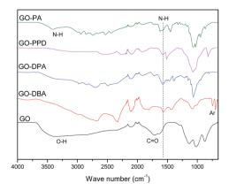
Fig. 5 FTIR spectra for GO, GO-DBA, GO-DPA, GO-PPD and GO-PA.
