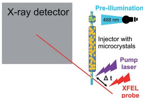
Fig. 1 Experimental setup of a time-resolved pump probe experiment to study photo-switching in a fluorescent protein.<sup>48</sup>
