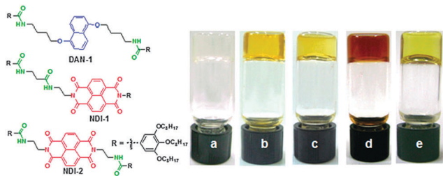
Fig. 3 (left) Structure of the gelators used by Das and Ghosh. 18 DAN-1 and NDI-1 form a self-sorted mixture, whilst DAN-1 and NDI-2 specifically co-assemble. (right) Photos of gels in methylcyclohexane formed by DAN-1 (a), NDI-1 (b), DAN-1 + NDI-1 (c), DAN-1 + NDI-2 (d) and NDI-2 (e). Reproduced from ref. 18 with permission from The Royal Society of Chemistry.
