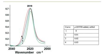
Fig. 1 Unsymmetrical hypsochromic broadening (ca.  $\sim$ 4 cm<sup>-1</sup> half-width) of the  $\nu$ (CO) band at 2019 cm<sup>-1</sup> as a result of gradual addition of p-DITFB to a 0.025 mmol cyclohexane solution of CpFe(CO)<sub>2</sub>TePh.
