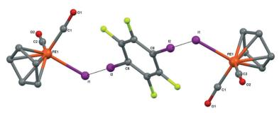
Fig. 7 Crystal structure diagram of 5, showing its I–I halogen-bonded trimolecular assemblies (CpFe(CO)<sub>2</sub>I)<sub>2</sub>( $\mu_2$ -DITFB). Hydrogen atoms are omitted for clarity. Selected distances (Å): Fe(1)–I(1), 2.6025(4); I(1)–I(2), 3.5488(3). Selected angles (°): Fe(1)–I(1)–I(2), 89.06(1); C(8)–I(2)–I(1), 175.50(7). Dotted lines link I atoms at a distance shorter than the sum of I–I vdW radii. 18
