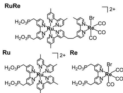
Chart 1 Structures and abbreviations of the Ru(II)–Re(I) supramolecular photocatalyst (**RuRe**) and its model mononuclear metal complexes used as the photosensitizer unit (**Ru**) and the catalyst unit (**Re**).
