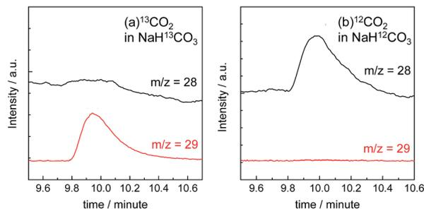
Fig. 5 GC-MS chromatograms of the gas products in the reaction chamber after irradiation (the detected  $m/z = 28$  for  $^{12}\text{CO}$  and  $29$  for  $^{13}\text{CO}$ ). The **RuRe**/CuGaO<sub>2</sub> photocathode was irradiated at  $\lambda_{\text{ex}} > 460$  nm in an aqueous solution containing 50 mM sodium bicarbonate (pH 6.6) at  $-0.7$  V vs. Ag/AgCl for 5 h using  $^{13}\text{CO}_2$  and NaH $^{13}\text{CO}_3$  (a) and ordinary  $\text{CO}_2$  and NaHCO<sub>3</sub> (b).
