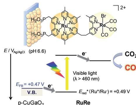
Fig. 3 Reaction scheme of the reduction of  $\text{CO}_2$  by the **RuRe/CuGaO<sub>2</sub>** hybrid photocathode.
