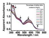
Fig. 5 UV-vis absorption spectra of 1 in CH<sub>2</sub>Cl<sub>2</sub> at 298 K upon increasing the diethyl ether content from 10 to 100% ([Pt]  $\approx 1 \times 10^{-5}$  M).
