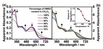
Fig. 4 (a) UV-vis absorption spectra of 1 in  $CH_2Cl_2$  at 298 K upon increasing the DMSO content from 10 to 100% ([Pt]  $\approx 1 \times 10^{-5}$  M). (b) UV-vis absorption spectra of 1 in DMSO upon cooling from 360 to 298 K ([Pt]  $\approx 1 \times 10^{-5}$  M). The apparent absorbance values have been obtained by correcting to a 1 cm path length equivalence.
