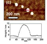
Fig. 6 (a) TEM and (b) SEM images prepared from a 300  $\mu$ M solution of 1 in DMSO on carbon-coated copper grids. (c) Tapping mode AFM image of 1 showing aggregates on silica wafers; bottom: height profile observed along the red line shown.
