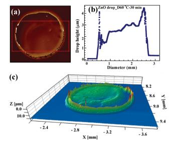
Fig. 11 ZnO drop dried at  $100\,^{\circ}\text{C}$  for 30 min in a hot air oven. (a) Optical image shows the presence of large sized cracks in the drop, (b) line profile of the dried drop (from the red dotted region marked in (a)) shows material accumulation and consequent ring formation at the edges. (c) The 3D profile of the drop shows the non-uniform thickness profile. The crack is also visible in the 3D profile. The colour represents the height variation.
