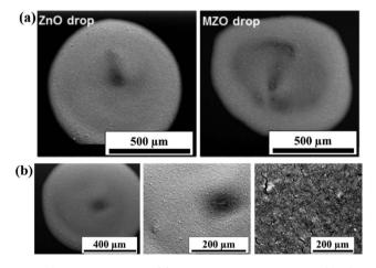
Fig. 14 SEM micrograph of (a) PZ5 and MZ1 drop dried at  $60\,^{\circ}\text{C}$  for 30 min. (b) Higher magnification images of PZ5 drop dried at  $60\,^{\circ}\text{C}$  for 30 min shows good particle connectivity, despite the presence of micro cracks.
