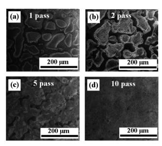
Fig. 6 SEM micrograph of commercial inkjet printed multi-pass patterns, using PZ4 ink, annealed at 200 °C for 3 h, (a) 1 pass (b) 2 pass (c) 5 pass and (d) 10 pass. Increased number of passes has improved continuity and annealing has caused fusion of the ZnO particles, showing a connected structure.
