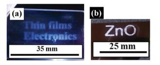
Fig. 7 Printed patterns of PZ4 ink at room temperature and annealed at 200  $^{\circ}$ C for 3 h. (a) 'Thin films' is printed in 5 passes and 'Electronics' in 10 passes on soda lime glass slide. (b) 'ZnO' pattern is printed in 10 passes on silicon wafer. Both patterns are continuous. The pattern was dried between individual passes using a hot air blower.
