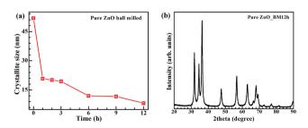
Fig. 2 (a) Crystallite size reduction as a function of milling time. After 10 h, the reduction in size is minimal. Hence, we have restricted the milling time to 12 h. (b) XRD of ball milled zinc oxide powders after 12 h. The particles are crystalline with peak broadening due to size reduction. The crystallite size is calculated from the XRD pattern using Debye-Scherrer formula
