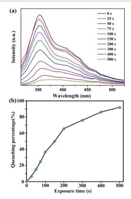
Fig. 4 Time-dependent emission spectra (a) and the corresponding luminescent quenching percentage (b) after exposure of 1 to NB vapour at room temperature.
