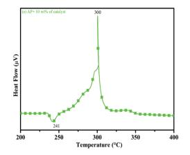
Fig. 15 DTA curve of AP modified with 10 w% catalyst.
