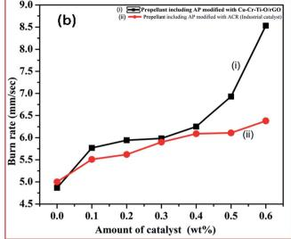
Fig. 17 (a) Images of the strand burner. (b) Burn rate of (i) SCP having AP modified with synthesized catalyst and (ii) SCP having AP modified with industrial catalyst.
