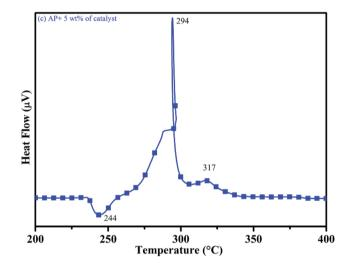
Fig. 13 DTA curve of AP modified with 5.0 wt% of catalyst.
