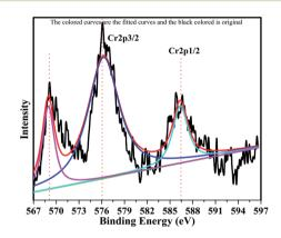
Fig. 7 XPS Pattern of chromium with fitted curves.
