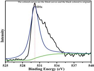
XPS pattern of oxygen with fitted curves.
