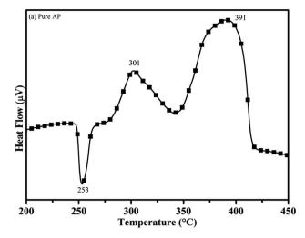
Fig. 11 DTA curve of pure ammonium perchlorate (AP).
