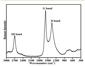
Fig. 3 Raman spectrum of the synthesized catalyst.
