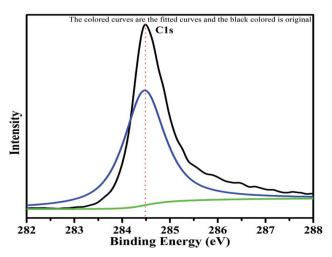
Fig. 10 XPS pattern of carbon with fitted curves.
