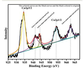
Fig. 6 XPS Pattern of copper with fitted curves.
