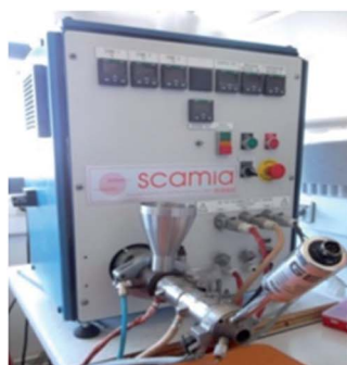
Fig. 7 Representation of a single-screw extruder.
