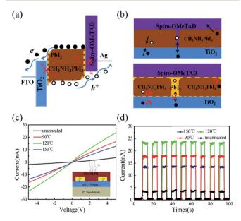
Fig. 7 Schematic diagram of (a) band gap of perovskite, Pbl<sub>2</sub> and perovskite device after passivation, (b) electrons and holes transfer process in the pristine and passivated perovskite film. (c) The currentvoltage (I-V) and (d) current-time (I-t) characteristic curves of the perovskite film annealed at different temperatures on the Si substrates under illumination (650 nm,  $1 \text{ mW cm}^{-2}$ ).
