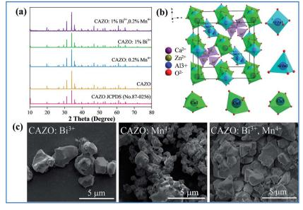
Fig. 1 (a) XRD patterns of the as-prepared phosphors CAZO:0.2%  $Mn^{4+}$ , CAZO:1%  $Bi^{3+}$  and CAZO:1%  $Bi^{3+}$ ,0.2%  $Mn^{4+}$  and the standard data for CAZO (JCPDS No. 87-0256) shown as a reference. (b) Crystal structure of the CAZO unit cell viewed in the c-direction and the coordination environment of the cation  $Ca^{2+}$  sites in CAZO. (c) The SEM images of CAZO:0.5%  $Bi^{3+}$ , CAZO:0.2%  $Mn^{4+}$  and CAZO:0.5%  $Bi^{3+}$ ,0.2%  $Mn^{4+}$ .
