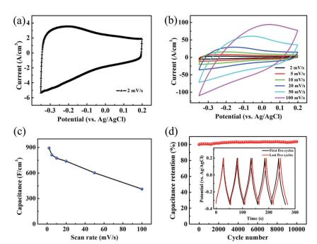
Fig. 5 The results of TCTL-II (a) at a scan rate of 2 mV s $^{-1}$ , and (b) at different scan rates. (c) Volumetric capacitance as a function of scan rate. (d) The cycling performance of the TCTL-II electrode at a current density of 5 A g $^{-1}$ . The black and red GCD voltage profiles of the TCTL-II electrode shown in the inset represent the first five cycles and the last five cycles, respectively.
