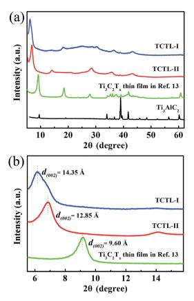
Fig. 2 (a) XRD patterns of the TCTL-I, TCTL-II, the previous  ${\rm Ti_3C_2T_x}$  thin film in ref. 13, and  ${\rm Ti_3AlC_2}$  powder and (b) the corresponding enlarged XRD patterns.
