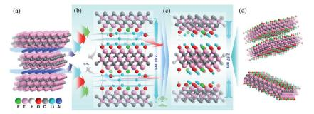
Fig. 4 Schematic diagram of the structural formation mechanism for the  $Ti_3C_2T_x$  sample. The atomic structure was built along the [110] direction. Atomic arrangements of (a) the  $Ti_3AlC_2$  structure, (b) the as-synthesized  $Ti_3C_2T_x$ -Li sheets, (c) storing in air for 50 days, and (d) one and two layers structures.
