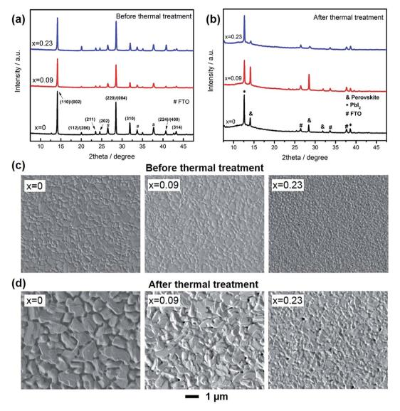
Fig. 2 Structure analysis of perovskite films. (a, b) XRD patterns for  $Cs_xMA_{1-x}Pbl_3$  before and after thermal treatment. (c, d) Top-down view SEM images of perovskite films before and after thermal treatment.
