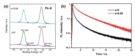
Fig. 4 (a) XPS study of Pb4f for x = 0 and 0.09 films. (b) Transient PL spectra for perovskite films with different Cs content.
